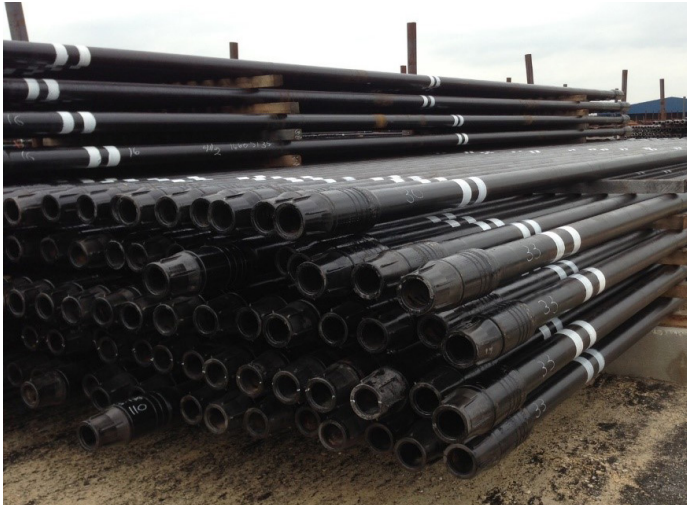
Drilling Pipes According to API 5DP specification levels PSL-1, PSL-2 and PSL-3 Grades: E-75, X-95, G-105 and S-135
