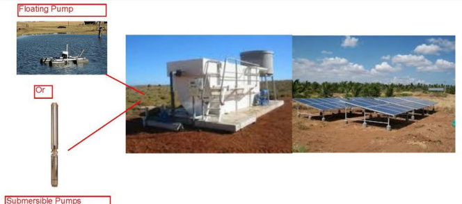
Solar Power Driven Water Treatment Plants • Capacities up to 40 m 3 / 8 hrs
