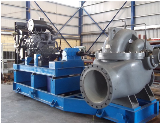
1 m 3 /Sec Horizontal Split Case Pump Set
