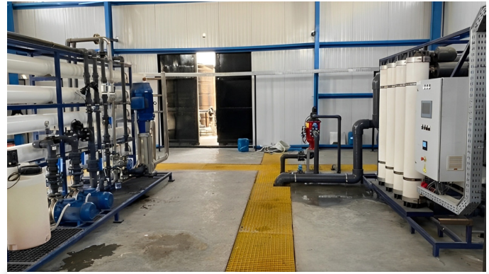
Sulfate Ground Water RO Plant
