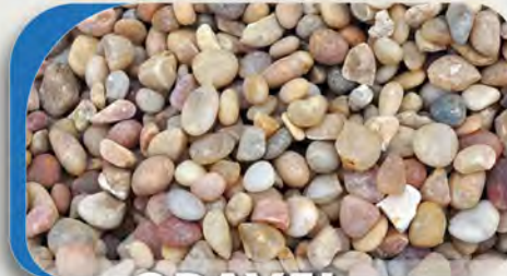
Filter Media (Silica Gravel)
