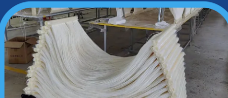
Membrane Bioreactor (MBR)
