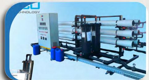
Reverse Osmosis Systems (RO)
