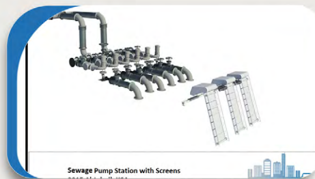
Sewage Pump Station with Screens
